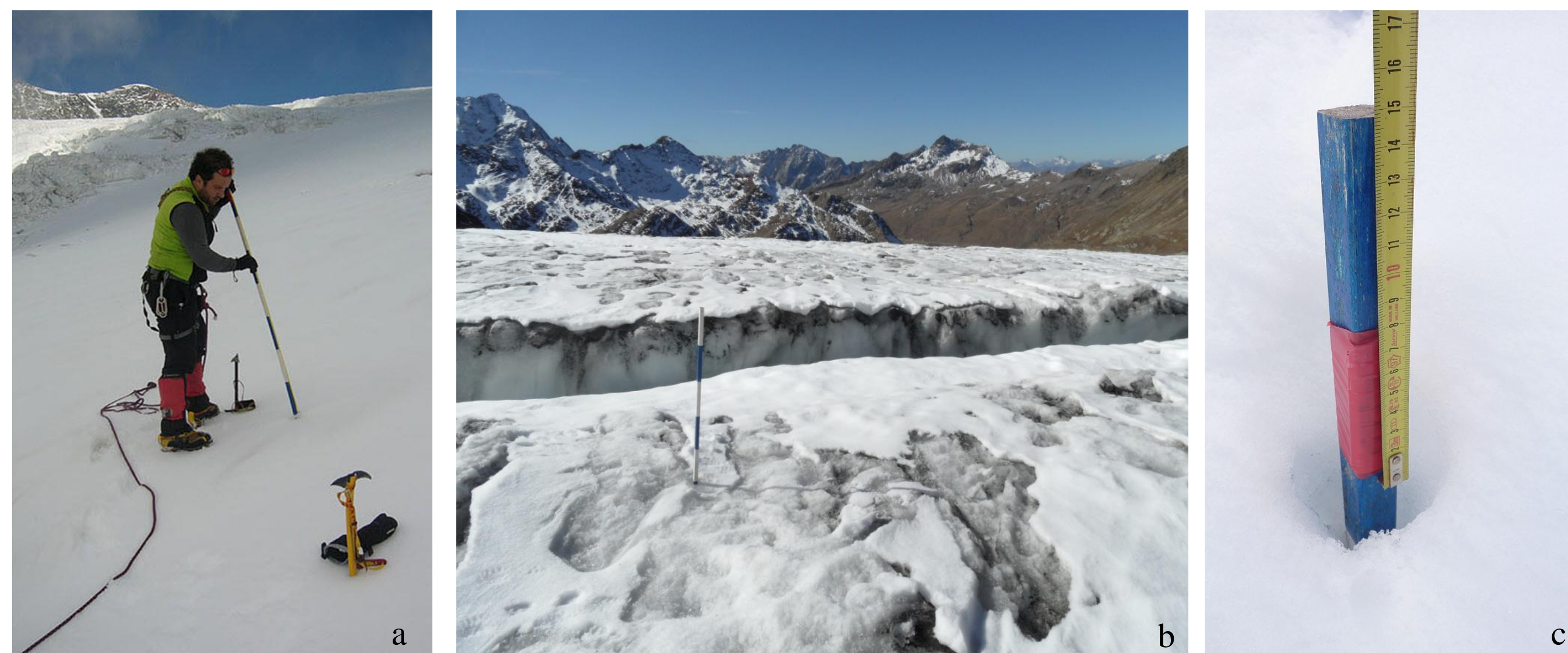
Fig. 1: ablation stake measurements on Fellaria glacier (a), and Dosegù glacier (b,c). (Photographs P. Pagliardi and L. La Barbera – SGL)
